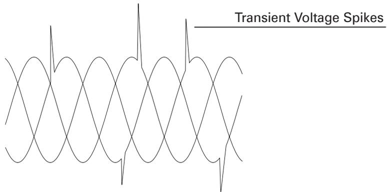
The most damaging voltage spikes are caused by lightning strikes. Although lightning strikes on high voltage lines are generally dissipated by utility transmission and arresters, a lightning strike on a power line several miles away still has the potential to cause extensive electrical damage. Damage to expensive electrical equipment can be either instantaneous or cumulative.
