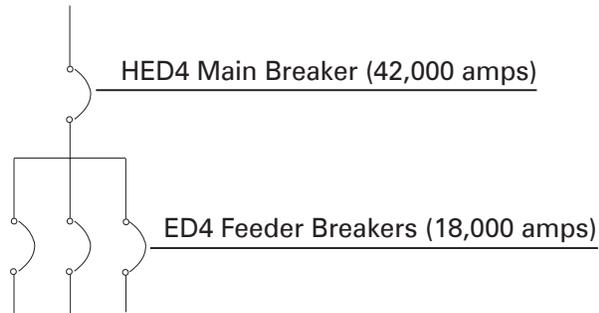
Series-rated breaker combinations must be tested in series in order to be UL listed. Siemens series-rated breakers are listed in the UL "Recognized Components Directory" (yellow books) Volume 1. Selected series-rated breakers are listed in the Speedfax catalog. Your Siemens sales engineer can provide more information on Siemens series-rated circuit breakers.
