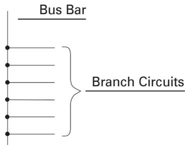
Bus bars are required to have phases in sequence so that an installer can have the same fixed phase arrangement in each termination point in any panelboard or switchboard. This is established by NEMA (National Electrical Manufacturers Association). It is possible to have a non-NEMA phase sequence which would have to be marked on the panelboard. It is assumed that bus bars are arranged according to NEMA. The following diagram illustrates accepted NEMA phase arrangements.
