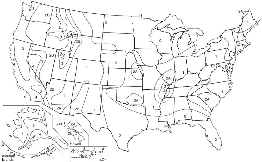
Siemens panelboards have undergone extensive seismic testing in order to obtain third party certification. Siemens panelboards will operate in zones 0, 1, 2A, and 2B with no modification. Panelboards that require zone 3 and 4 ratings are available with standard lead times.
