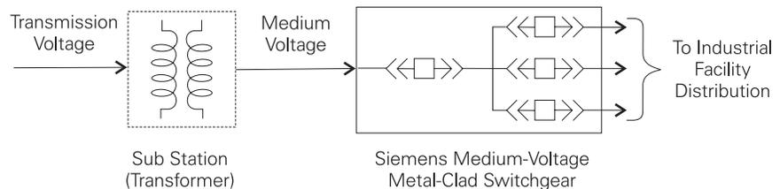
It can be seen in this example that one 38 kV metal-clad switchgear unit is supplying power to two 5 kV metal-clad switchgear units and one 15 kV metal-clad switchgear unit. This is one way power might be distributed throughout a large industrial complex made up of several buildings, each requiring great amounts of electrical power.
