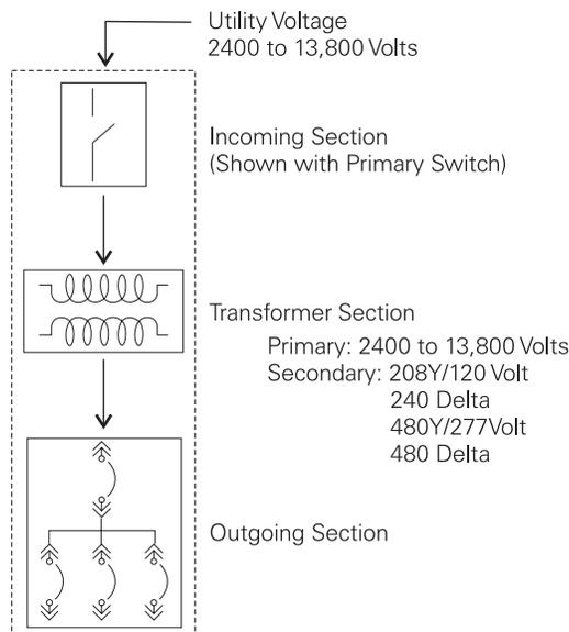
A primary switch is used to provide a means to connect and disconnect the secondary unit substation from the supply service. The transformer section can be liquid filled, ventilated dry type, or a cast-coil type. The outgoing section can be a Siemens Sentron switchboard, such as the RCIII, or Type R low-voltage switchgear.
