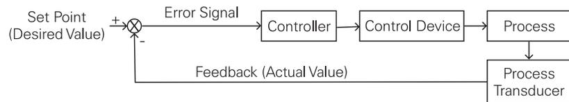
A variety of approaches can be used for process control depending upon the complexity of the process being controlled. A small batch process often lends itself well to control by one PLC or a few networked PLCs. A representation of the process showing its current status and a history of data recorded at various points in the process is often provided to an HMI system networked to the PLCs.
