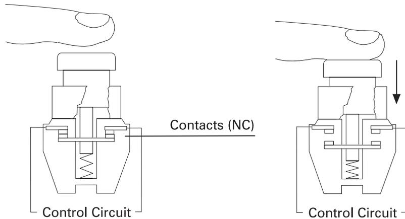
Pushbuttons are available with variations of the contact configuration. For example, a pushbutton may have one set of normally open and one set of normally closed contacts so that when the button is depressed, one set of contacts is open and the other set is closed. By connecting to the proper set of contacts, either a normally open or normally closed situation exists.
