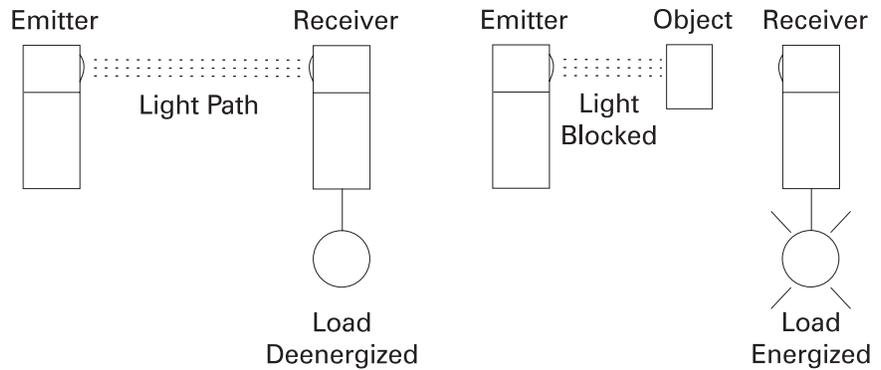
Light operate is an operating mode in which the load is energized when light from the emitter reaches the receiver.
