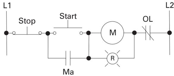
When the coil is energized, the light will illuminate to indicate the motor is running. In the event the pilot light burns out the motor will continue to run.
