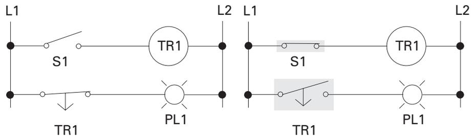
When S1 is opened, timing relay TR1 is deenergized. After 5 seconds, the associated normally closed contacts close, illuminating PL1.
