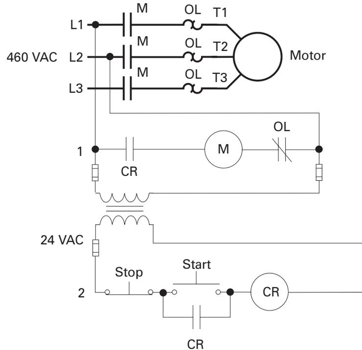
When the "Start" pushbutton in line 2 is momentarily depressed, power is supplied to the control relay (CR).
