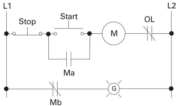
Depressing the “Start” pushbutton and energizing the “M” contactor opens the normally closed “Mb” contacts, turning the light off.
