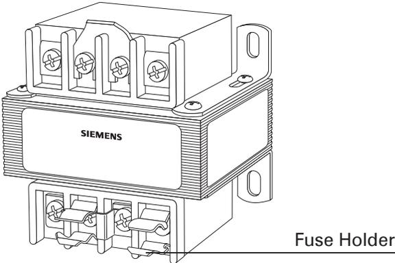
In the following example, the power circuit is 460 VAC. A control transformer is used to step the voltage down to 24 VAC for use in the control circuit. The electromagnetic coil voltage must be rated for 24 VAC. Fuses on the primary and secondary windings of the transformer provide overcurrent protection.
