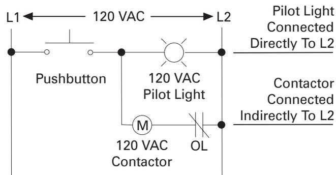
Control loads are generally not connected in series. The following illustration shows two ways to connect a control load. In one instance the control loads are improperly connected in series. When the pushbutton is depressed, the voltage across L1 and L2 is divided across both loads, the result being that neither load will receive the full 120 volts necessary for proper operation. If one load fails in this configuration, the entire circuit is rendered useless.
