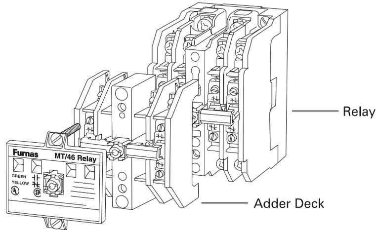
Class 46 machine-tool relay contacts can be field changed between normally open (NO) and normally closed (NC).
