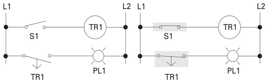
When S1 is opened, TR1 begins timing. When 5 seconds has elapsed, TR1 will open its associated normally open contacts, extinguishing pilot light PL1.
