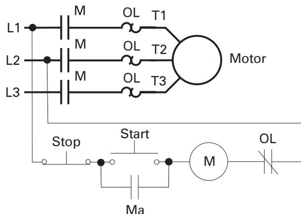
Momentarily depressing the "Start" pushbutton completes the path of current flow and energizes the "M" contactor's electromagnetic coil.
