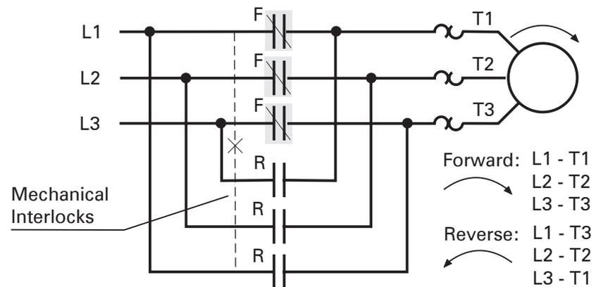
When the "R" contacts are closed, current flows through the motor in the opposite direction causing it to rotate in a counterclockwise direction. Mechanical interlocks prevent both forward and reverse circuits from being energized at the same time.
