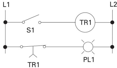
When S1 is closed, timing relay TR1 is energized. After a timed delay of 5 seconds, the associated normally closed TR1 contacts open, extinguishing PL1. When S1 is open, deenergizing TR1, the TR1 contacts close immediately, illuminating PL1.
