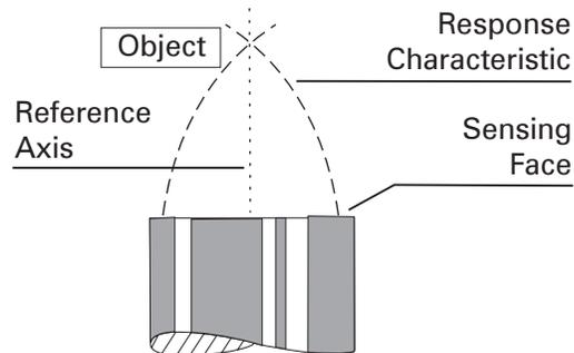
The point at which the proximity switch recognizes an incoming object is the operating point. The point at which an outgoing object causes the device to switch back to its normal state is called the release point. The area between these two points is called the hysteresis zone.
