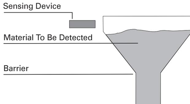
The following chart illustrates the proper capacitive proximity switch when detecting material through a barrier.
