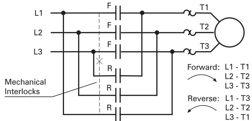
When the "F" contacts are closed, current flows through the motor causing it to turn in a clockwise direction.
