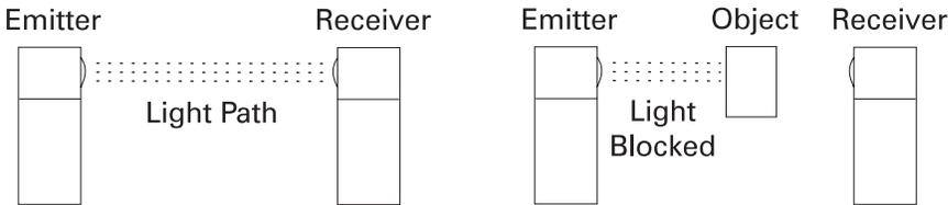
A photoelectric sensing device, for example, might be positioned over a roll of paper. When the roll on the winder reaches a predetermined diameter, it will interrupt the light beam and automatically stop the motor.
