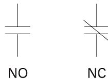
The standard method of showing a contact is by indicating the circuit condition it produces when the actuating device is in the deenergized or nonoperated state. For example, in the following illustration a relay is used as the actuating device. The contacts are shown as normally open, meaning the contacts are open when the relay is deenergized. A complete path of current does not exist and the light is off.
