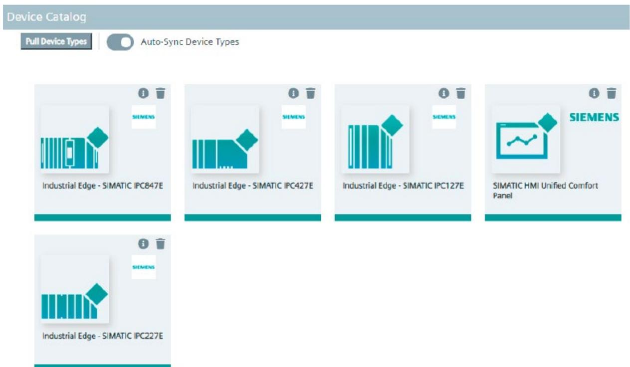
By clicking "Pull Device Types", you manually synchronize all published Edge Device Types from the IE Hub to the IEM. If you want to automatically synchronize the published Edge Device Types from the IE Hub to the IEM, enable the "Auto-Sync Device Types" toggle. If you do not want to automatically synchronize the published Edge Device Types from the IE Hub to the IEM, disable the toggle. In that case, you must manually synchronize the Edge Device Types to stay up to date.
