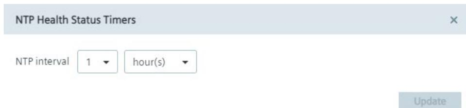
In this screen you set the monitoring interval in which the IEM-OS checks the NTP server status. By default, the interval is set to 1 hour. Maximum interval is 1 day and minimum interval is 1 minute. To save the changes, click "Update".
