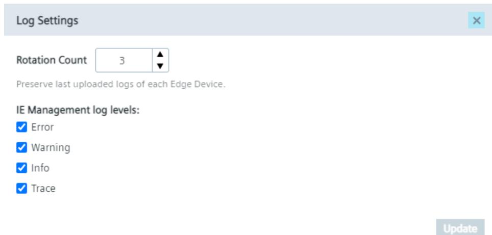
The "Rotation Count" setting manages the amount of log files of each Edge Device that are stored on the IEM. The IEM only stores the amount of the latest log files that you have set in this setting, by default 3 log files are getting stored. The rest will be removed automatically from the IEM.
