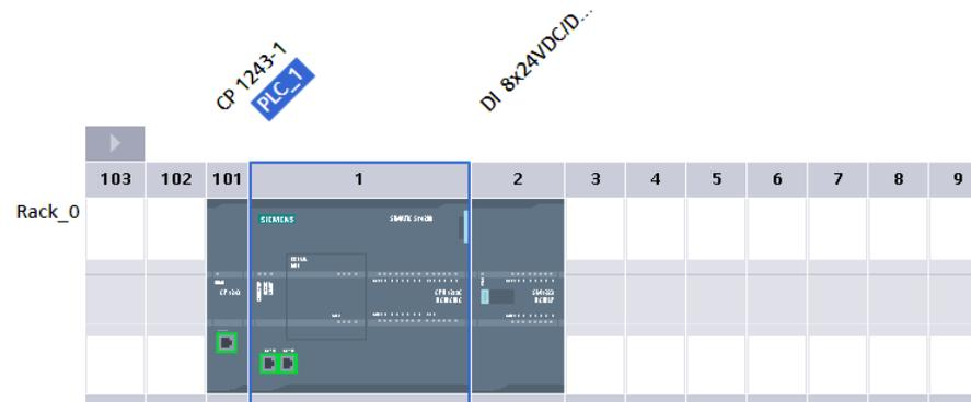
After a short delay, the S7-1200 and all local modules are added to the Project and are displayed in the work area of the “Devices and networks” editor.
